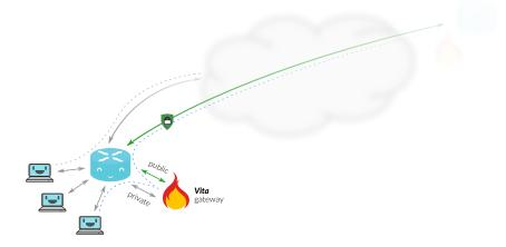
Vita is on its way to become an affordable, open, stand-alone solution to that problem. It is designed to play well with your existing routers, and can be deployed in a bump-in-the-wire or on-a-stick configuration. You can probably throw together a Vita box that handles 1-Gigabit Ethernet line rate at 64-byte packets for well under 500 Euro in parts (efficient software implementations go both ways!)
